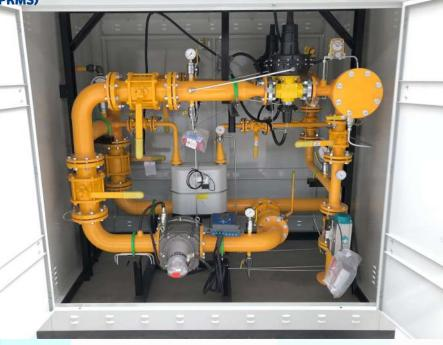
Kayamak, provides custom engineered Pressure Reduction and Metering Stations (PRMS) in accordance with EN 11672 to meet each customers' desired pressure range and gas flow apacity. PRMS are built to order including a range of gas regulators, slam-shut valves, gas filters, isolation valves, gas meters, & volume corrector.
